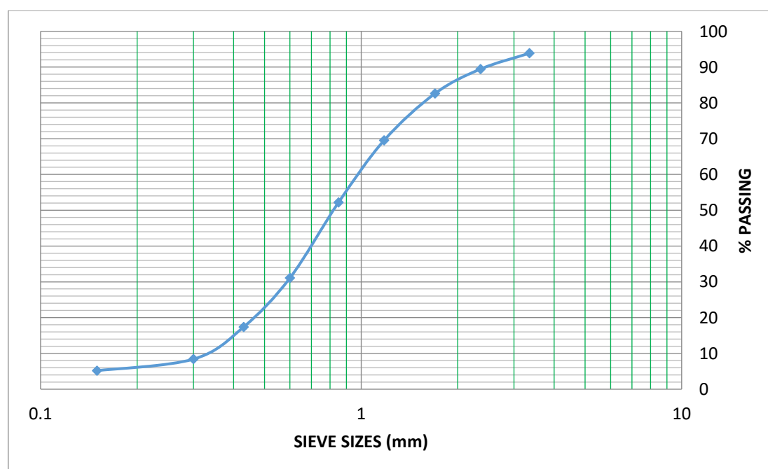
Figure 1: The Grading curve of the River Sand
